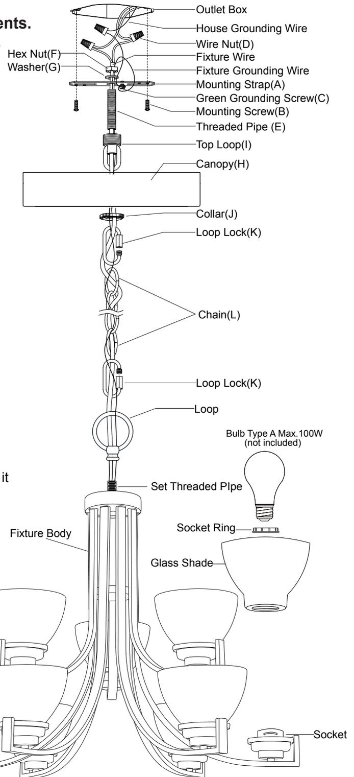
9. Pull out the source wires from the outlet box. Make wire connections using wire nuts as follows:
